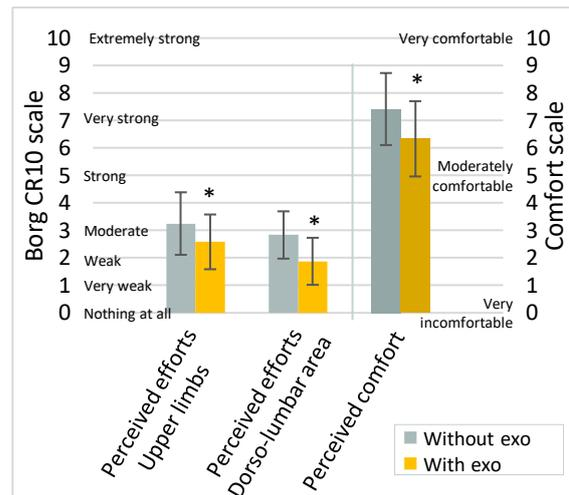
Figure 11: Subjective results for task 3: perceived efforts and perceived comfort with and without the exoskeleton. Asterisks denote significant differences ( $p < .05$ ) from the reference condition (without exoskeleton)
