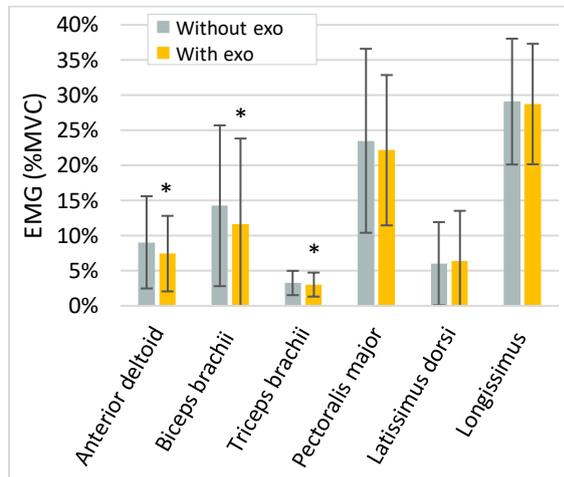
Figure 10: Mean EMG values normalized by the MVC for each muscle, with and without the exoskeleton. Asterisks denote significant differences ( $p < .05$ ) from the reference condition (without exoskeleton)
