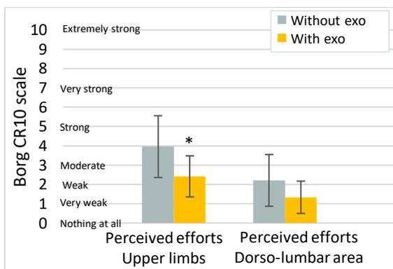
Figure 7: Subjective results for task 1: perceived efforts with and without the exoskeleton. Asterisks denote significant differences ( $p < .05$ ) from the reference condition (without exoskeleton)
