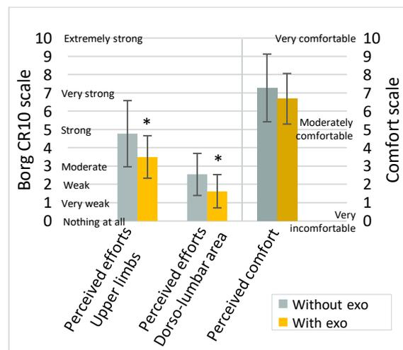
Figure 9: Subjective results for task 2: perceived efforts and perceived comfort with and without the exoskeleton. Asterisks denote significant differences ( $p < .05$ ) from the reference condition (without exoskeleton)
