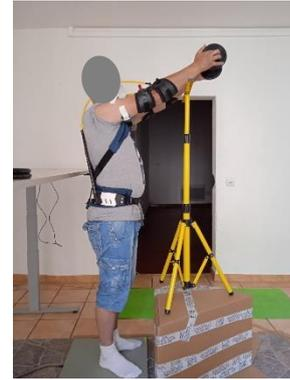
Figure 1: static task with arms at  $105^\circ$ , 1 kg per hand
