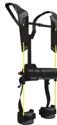
Figure 1: Isometric view of the HAPO. Elastic springs are represented in yellow
